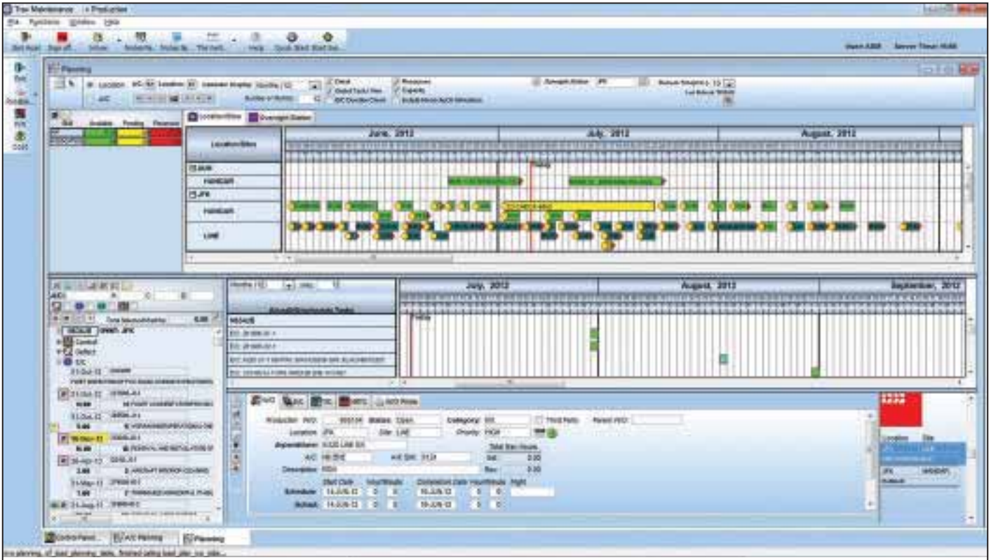
The 'TRAX Maintenance' user interface is designed to enhance the visibility of maintenance requirements through colour-coded displays which combine graphical and spreadsheet data.
